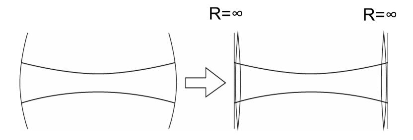
The elements between the plane mirrors now can be described by a single-pass ABCD matrix.
