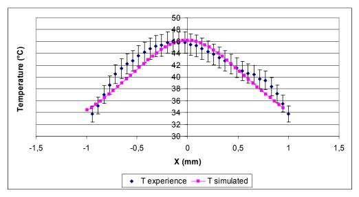
Figure 2. Measured and computed distribution of temperature T for Nd:YAG 1 at. % at the entrance plane of the pump beam.
