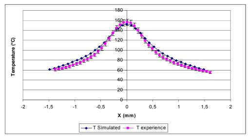
Figure 3. Measured and computed distribution of temperature T for  $Nd:YVO_4$  1 at. % at the entrance plane of the pump beam.
